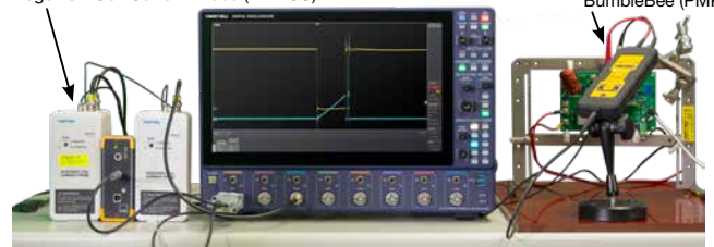
Measurement Example: Switching voltage / current of GaN Device evaluation board Rogowski Coil Current Probe (IWATSU) High Voltage Differential Probe BumbleBee (PMK)
