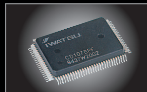
Specially-designed gate array with built-in CPU
